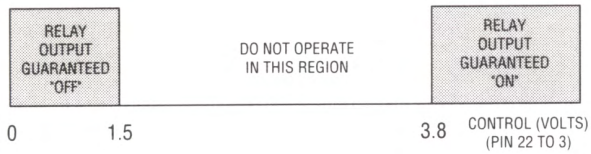
(B) 2 TERMINAL CONTROL RANGE
